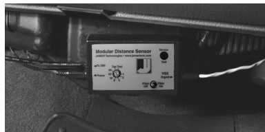
Fig. 2.3 MDS Mounted Under Dash
